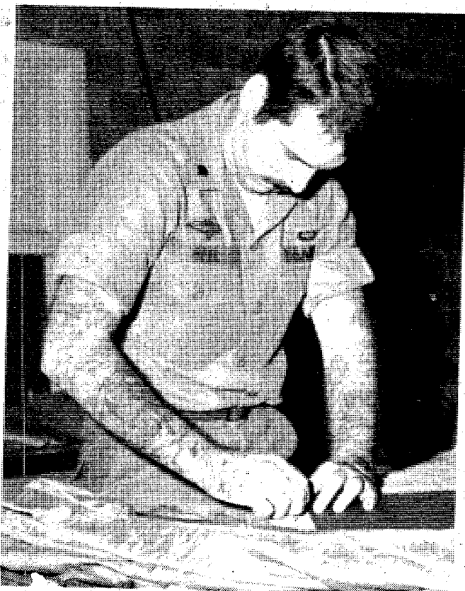
Sp4 Samuel Neal prepares a parachute for patching by basting down the cut edges at the rigger's maintenance shop.
